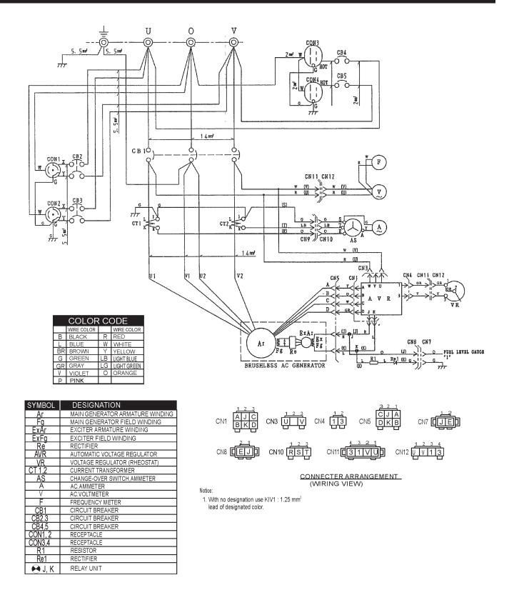
Figure 48. Generator Wiring Diagram
